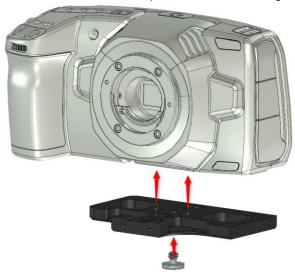
2. Attach the cage side to the base using 2X M4 screws, do not fully tighten the screws yet.
