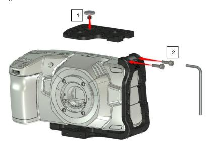
Open the cover of the HDMI socket in the camera, put the angled HDMI adapter in the HDMI socket and attach the cover over the HDMI adapter using two M4 screws.
