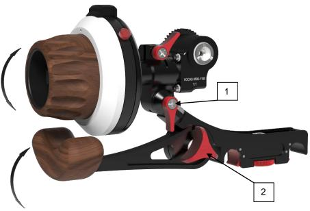
1. Loosen this red winged nut nr. 1 to release the gear unit and allow it to tilt in relation to the 15 mm snap-on bracket.
