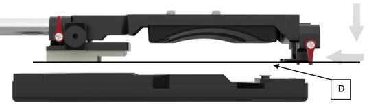
Double check: now try the base plate on a VCT-14 tripod plate, make sure the front of the base plate attaches correctly, and the wedge of the VCT-14 Clamping block grips the mushroom (at the rear) correctly.
