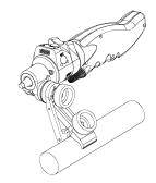
Also available is a panbar-clamper for mounting the ZiF in line with the panbar of your tripod.
